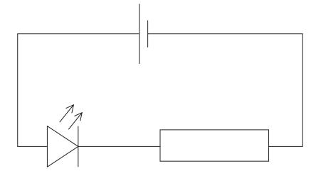
(a) Add meters to the diagram to measure the voltage of the resistor and the current in the resistor.
